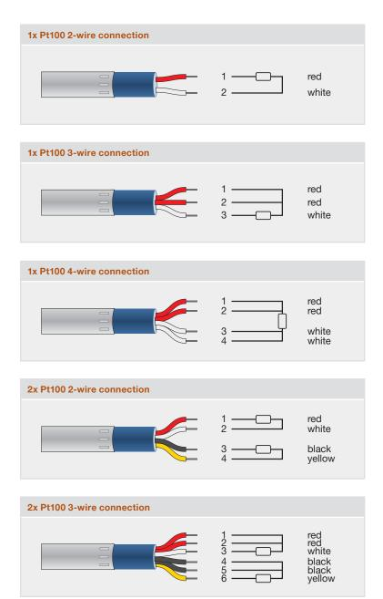
Depending on the connecting cable used, deviations in the conductor colours are possible, if the measuring circuits remain clearly assignable.
